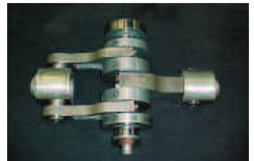
Couple-free, balanced design minimizes vibration and piping fatigue.
