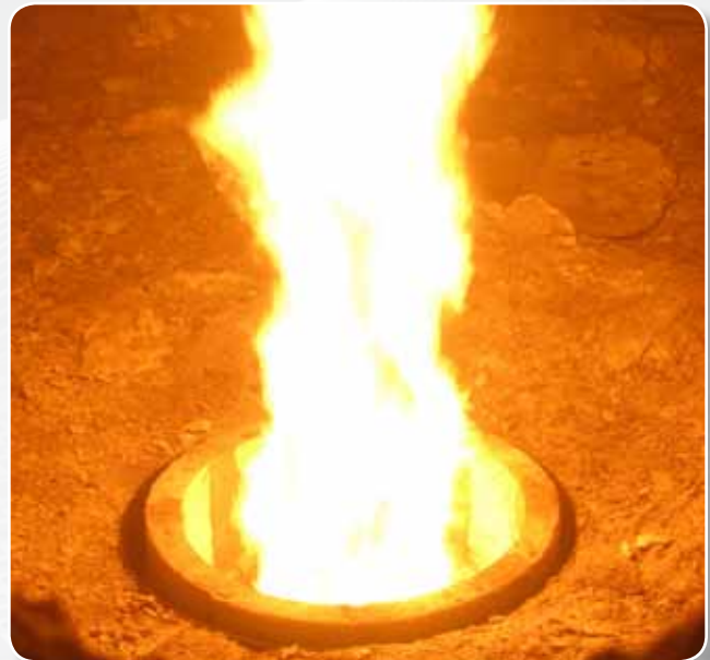
AK Staged Air Low Emissions Combination Burner Operating on Oil Only
